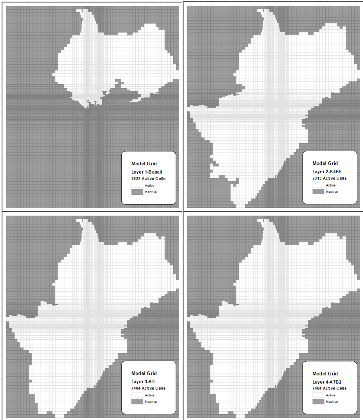
Figure 3-1. Numerical flow model grid for the Azraq Basin with variable spatial resolution. Panels show active cells for each model layer.
