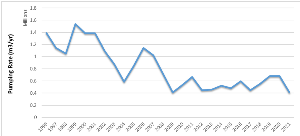
Figure 2-4. Rates of groundwater pumped from the MWI well to the wetland during the period 1996 – 2021.
